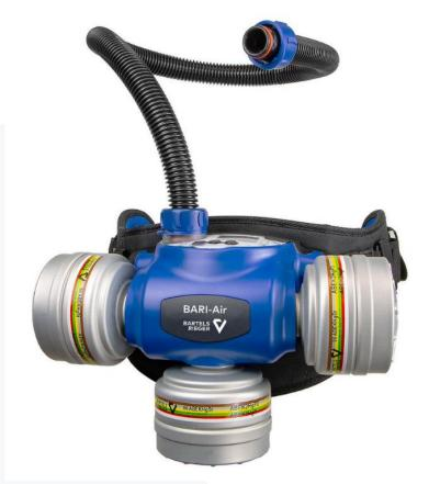
The blower filter unit filters the ambient air through three filters connected to the unit. Depending on the type of filter, the filters absorb particles, gases, vapors or combinations thereof from the ambient air. After the filtration process, treated ambient air is fed, through a hose, into the facepiece where it is available as breathing air. The positive pressure generated prevents pollutants from the environment from entering the headpiece.
